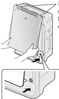
Push in the protrusion into holes (2 places) of product and press properly.
